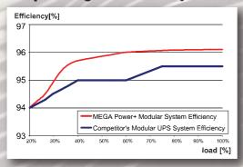
Webpro delivers the highest efficiency rate. At an efficiency rate of 96%, Webpro provides significant energy and cooling savings.
